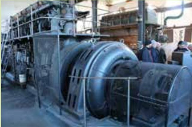
The six cylinder two stroke, Harland – Wolfe to the right of the photo and the six cylinder, four stroke **Paxman with it's alternator and excitor** are a sight and sound not to be missed when they fire into life!!
