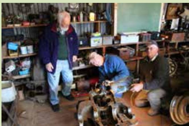
With some help from Ian Le Grice and Graeme Shefford , John Neal removes the last set of gears so the transmission case can be cleaned and inspected.
